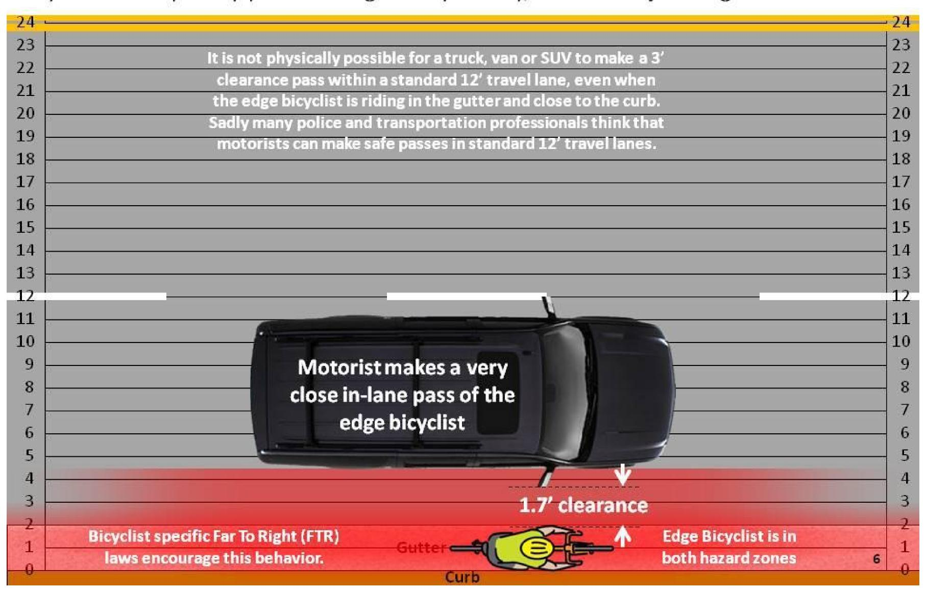
A bicyclist riding near the edge of a standard 12' wide travel lane, in this case in the gutter, often seen on city streets, is in both the road edge and close pass hazard zones. Bicyclists riding in this uncomfortable way will be frequently passed, sometimes dangerously closely, and will also be subject to curb face, gutter seam and debris hazards.
