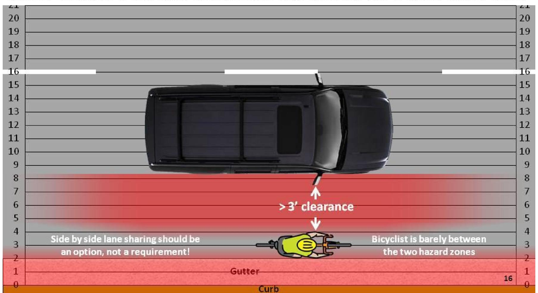
When the lane is 16' wide, a bicyclist riding can just barely avoid the close passing zone of trucks, SUVs and vans, as well as the edge hazards. This is a very narrow zone and not very comfortable.
