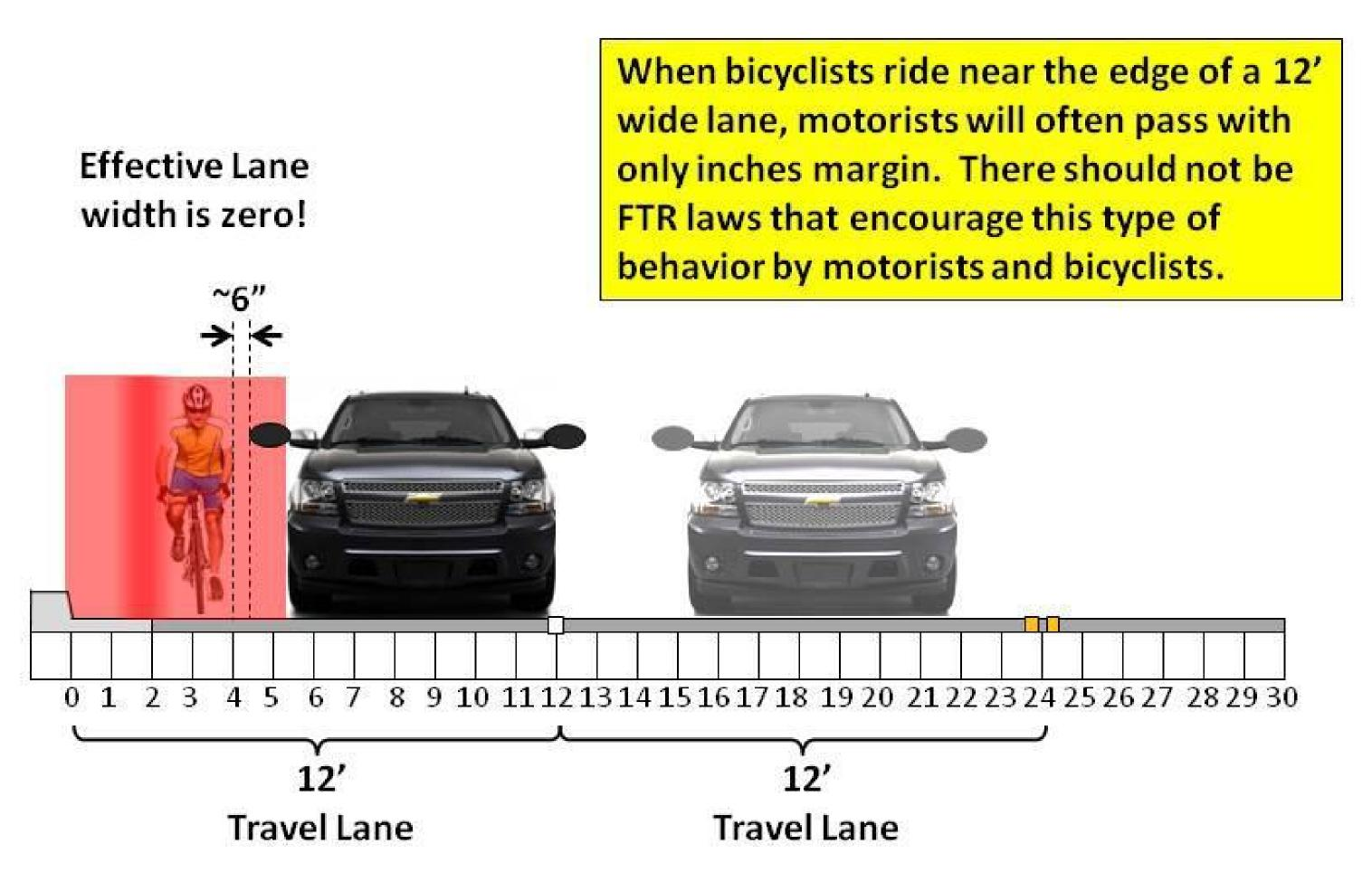
A bicyclist that controls the right hand lane is avoiding, by the maximum margin, both the close passing zone and the road edge hazard zone, and inhibits in-lane passing by overtaking motorists. This is why LCIs/CSIs teach cyclists to control narrow lanes.
