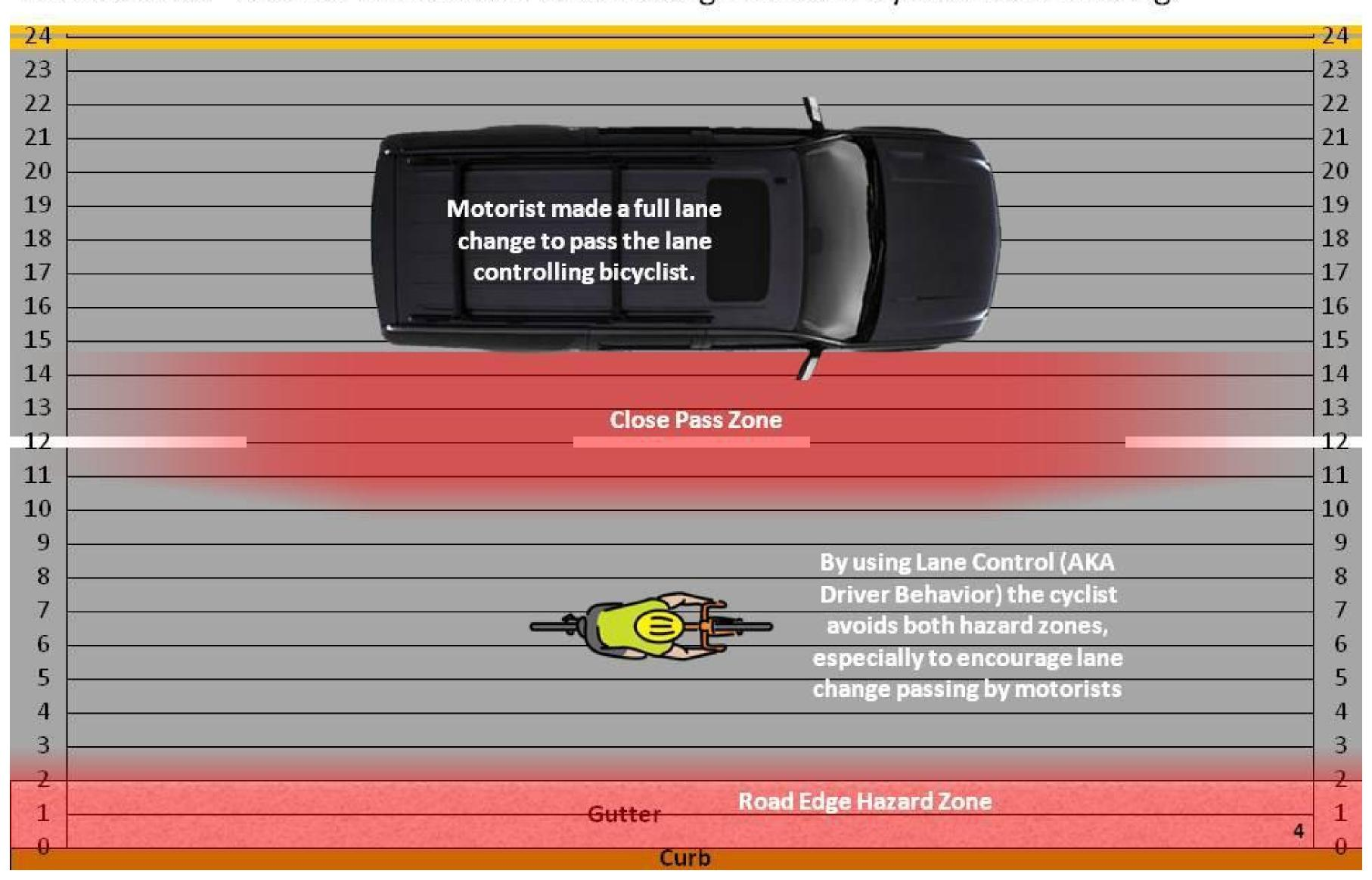
A 2 foot wide bicyclist that controls a standard 12' right hand lane is avoiding, by the maximum margin, both the close passing zone of motor vehicles in the adjacent lane as well as the road edge hazard zone. This 12' lane is NOT wide enough for side-by side lane sharing (see next slide).
