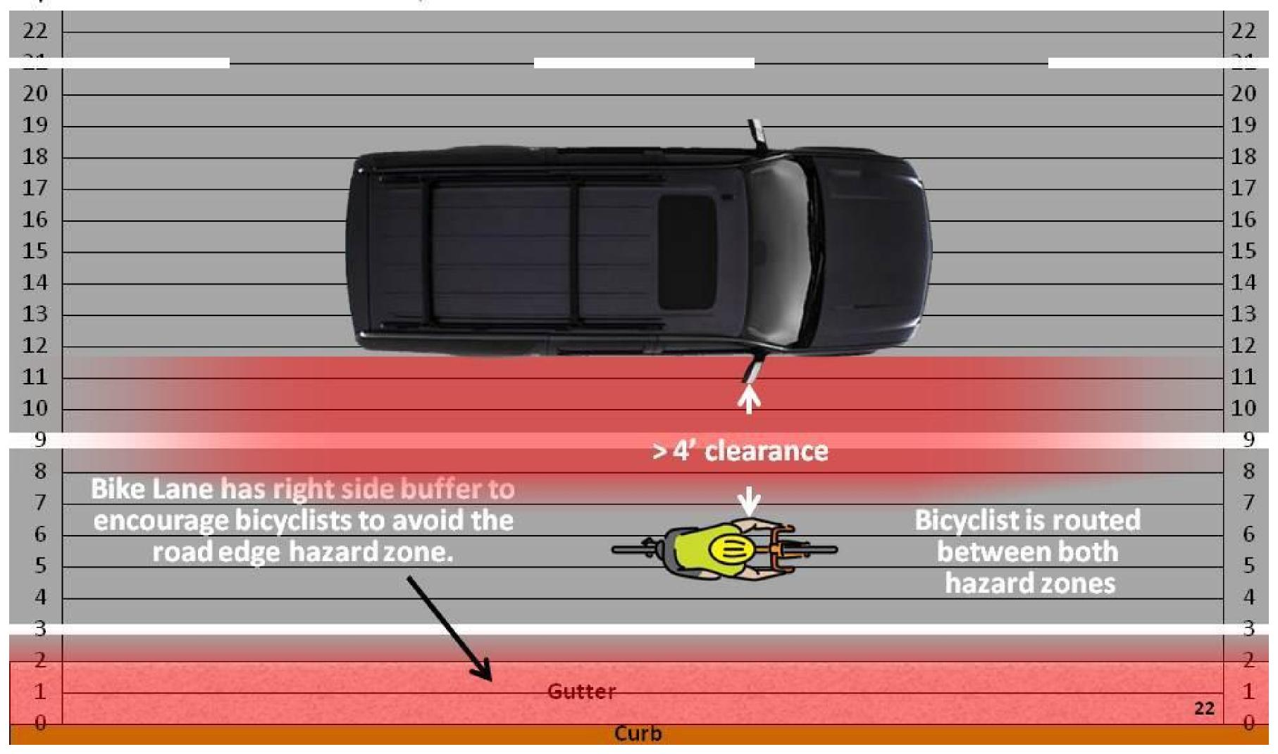
With 21' of width, a 12' travel lane can be striped adjacent to now 9' wide, right side buffered bike lane. Here the cyclist has ample enough room to avoid both the close passing zone of trucks, SUVs and vans, while the edge hazard is to the right of and completely outside the bike lane. A substantial amount of road width is required to create comfortable, hazard-free bike lanes.
