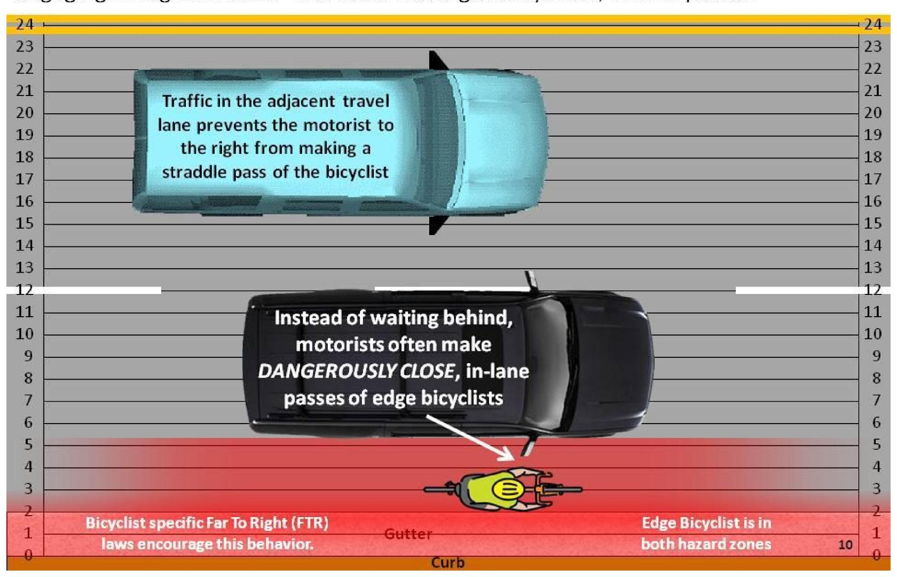
When traffic is in the adjacent lane, a motorist overtaking a bicyclist cannot make a straddle pass, and will often squeeze by within the same lane where the bicyclist is engaging in edge behavior. This leads to **DANGEROUSLY CLOSE**, in-lane passes as can be seen in this cross-section view.
