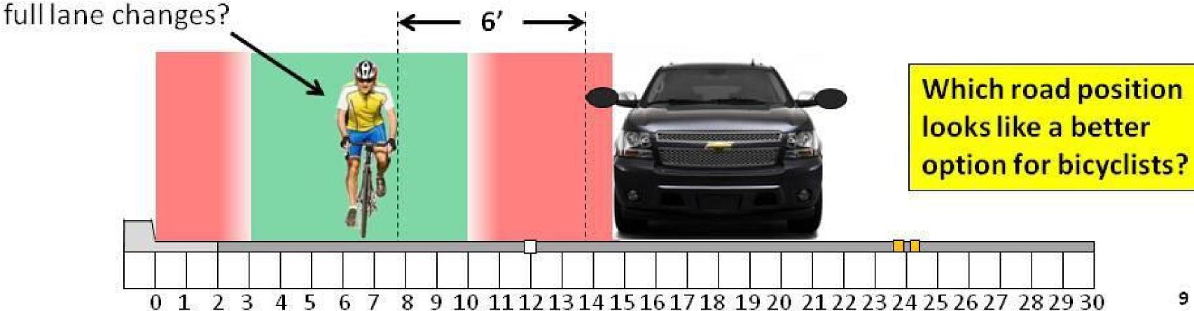
When traffic is in the adjacent lane, a motorist overtaking a bicyclist cannot make a straddle pass, and will often squeeze by within the same lane where the bicyclist is engaging in edge behavior. This leads to dangerously close, in-lane passes.
