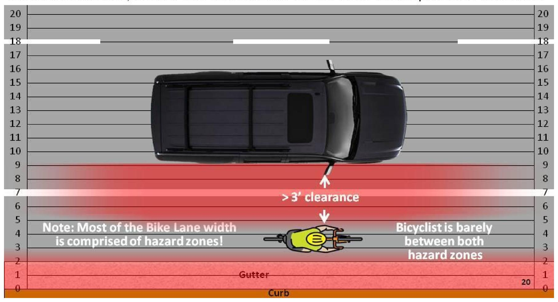
With 18' of width, an 11' travel lane can be striped adjacent to now 7' wide bike lane. Here the cyclist has just enough room to avoid both the close passing zone of trucks, SUVs and vans, and the edge hazards. It takes a substantial amount of road space to create comfortable, hazard-free bike lanes as we will show on the next slide.
