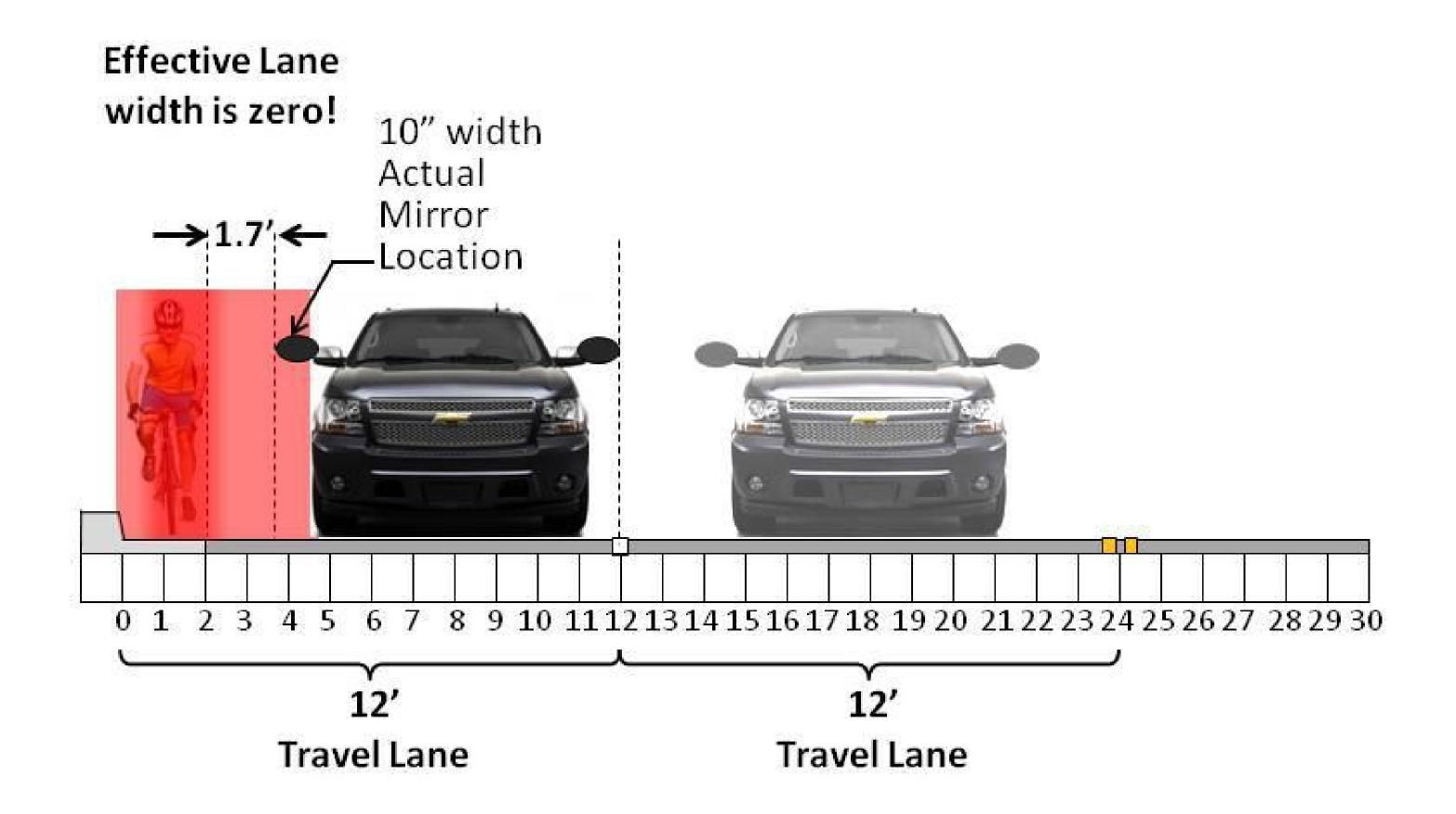
Often a motorist will straddle the lane line with their wheel tracks to pass a bicyclist engaged in edge behavior, instead of making a full lane change to pass. We call this a "straddle pass", and it is not as safe for the bicyclist as a full lane change pass.
