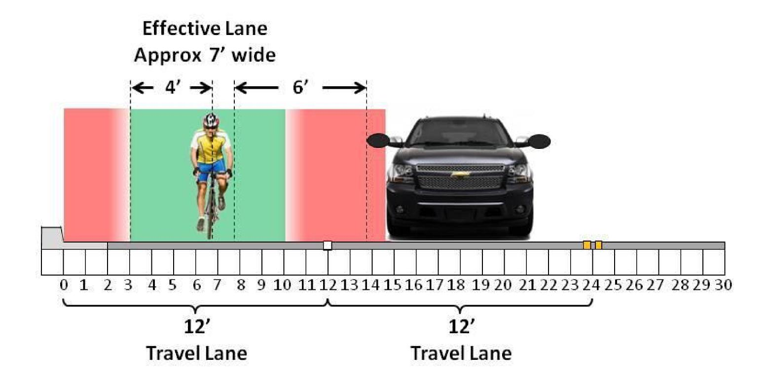
A bicyclist riding at the edge, in this case the gutter, often seen on city streets, is in both the road edge and close pass hazard zones. Bicyclists riding in this uncomfortable way will be frequently passed dangerously closely, and be subject to gutter hazards.
