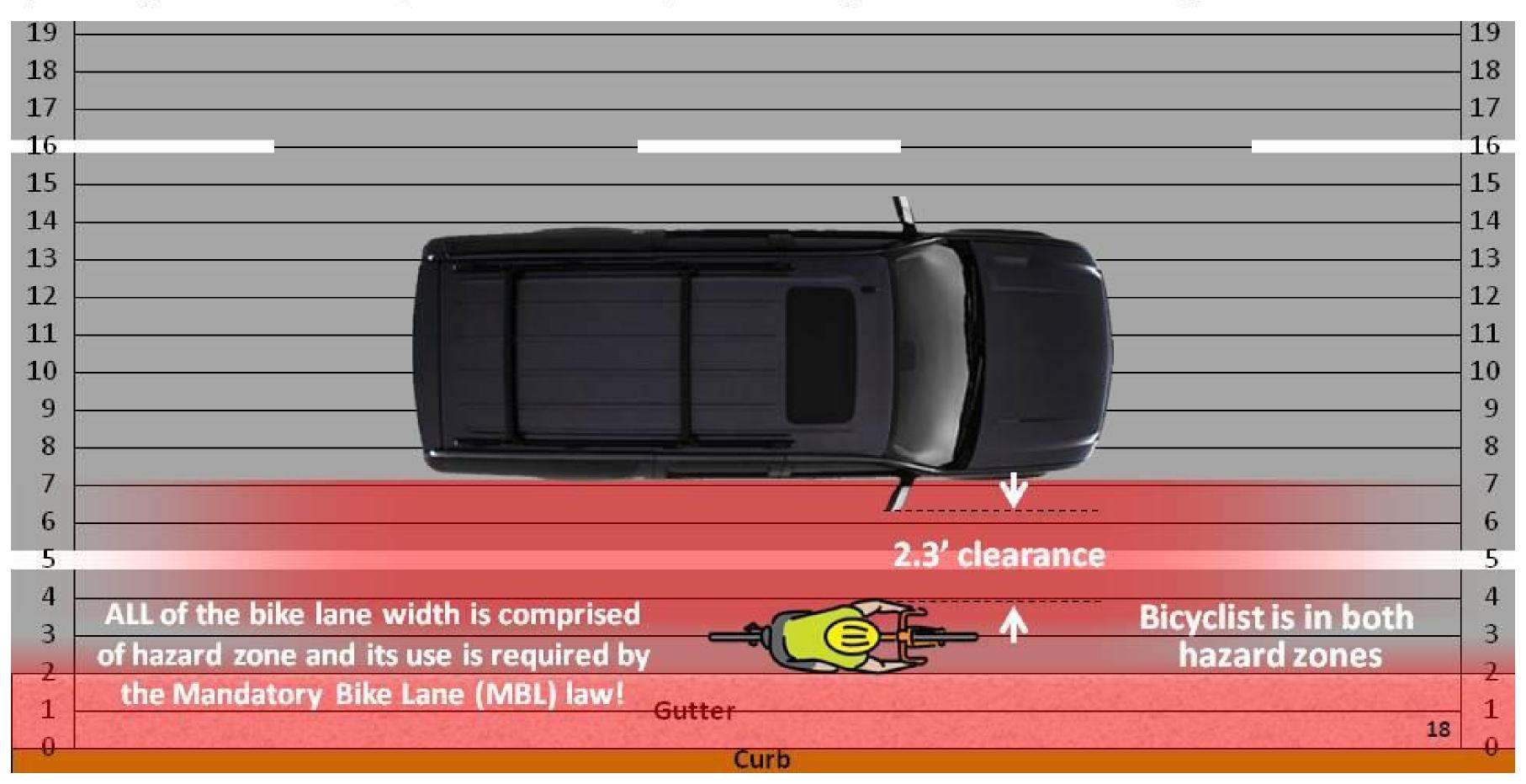
With that same 16' of available space, an 11' travel lane can be striped adjacent to a minimum standard 5' wide bike lane. The cyclist has to choose either the close passing zone of trucks, SUVs and vans, or the edge hazards. Is this a good choice for bicyclists?
