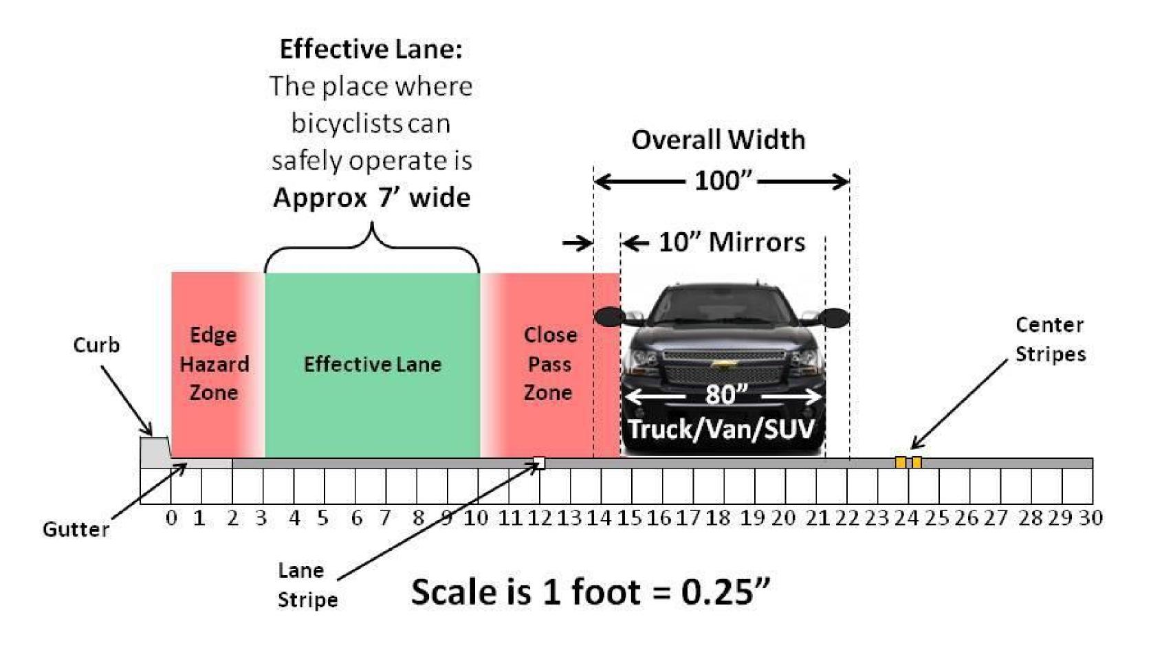
A bicyclist that controls the right hand lane is avoiding, by the maximum margin, both the close passing zone of motor vehicles in the adjacent lane as well as the road edge hazard zone. This 12' lane is NOT wide enough for side-by side lane sharing.
