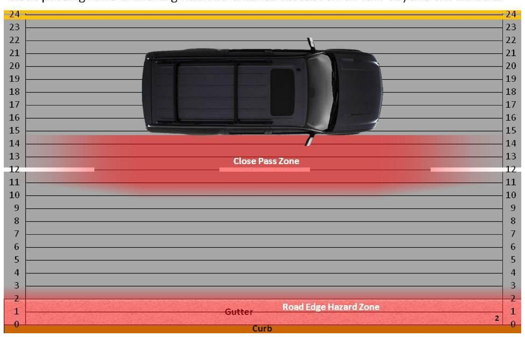
In this cross-section view, the hazard zones are displayed as vertical translucent red regions. The edge hazard zone includes all of the gutter as well as foot or so of clearance from the gutter seam. The close passing zone of moving vehicles extends at least three feet beyond the mirrors which in turn can and often do extend up to 10" beyond the side of vehicles. Not also the lane/center stripes.
